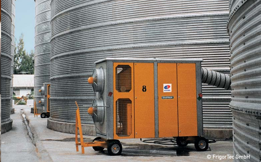
1 GRANIFRIGOR™ grain cooling in steel silos
